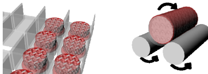
Figure 7.1: Schematic of static seeding (left) versus dynamic seeding (right). In the static seeding procedure, cell suspensions were pipetted on top of the scaffolds and left to stand for 4 h in an incubator. In the dynamic seeding procedure, the cell suspensions were pipetted on the scaffolds while sitting inside a syringe tube, followed by incubation on a roller (0.5Hz) for 4 h.
